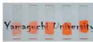
Hybrid films exhibiting very high TPA efficiencies. These films consist of a clay and a fluorescent dye.
