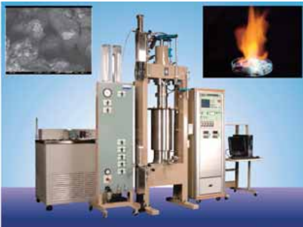
Figure 1. Triaxial testing apparatus for methane hydrate bearing soils
